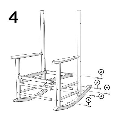
Position other Side Frame onto Braces and Seat Frame. Start five (5) (A) screws, but KEEP LOOSE.
