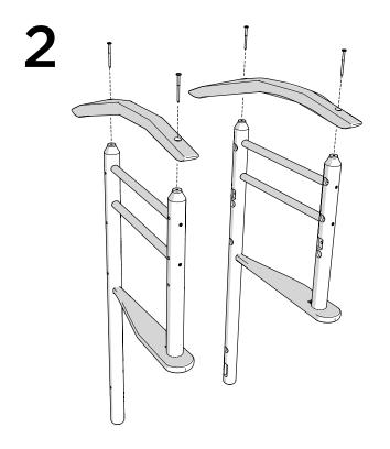
Flex of rocker bottoms may be required to line up screws with pilot holes.
