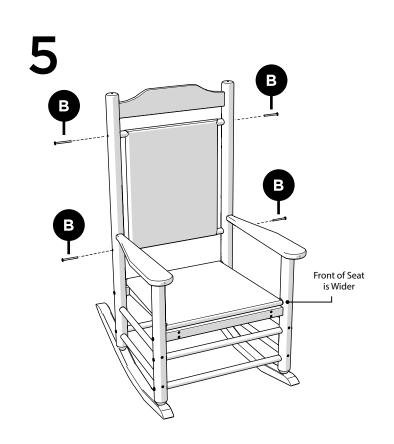
Place Seat Panel, Back Panel, and Head Piece in position. Start 4 B screws, but KEEP LOOSE.
