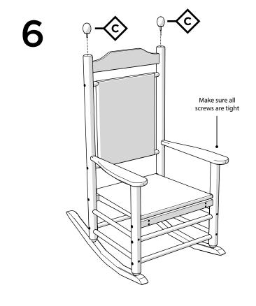
Attach Finials to tops of posts. Perform one last check to make sure all screws are tight.
