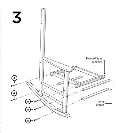
Attach Long Braces, Short Brace and Seat Frame to Side Frame using five (5) (A) screws.
