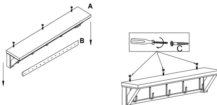
**NOTE:** It is recommended that the Hook Shelf be stud-mounted for stability. If unable to locate studs, you may need to use an alternative fastener for your application.
