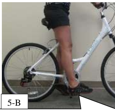
5-B To determine proper saddle height, position right pedal at the bottom of its revolution, aligned with the seat tube. While sitting on saddle, place your heel on right pedal. Your leg should be fully extended (5-B).
