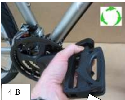
4-B Insert right pedal into right crankarm and turn clockwise.
