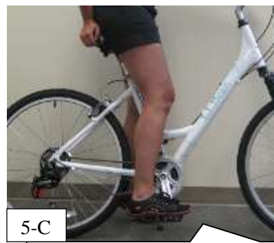
5-C Adjust saddle height if necessary and repeat. Now place the ball of your foot directly over the center of the pedal (normal riding position). This should result in the correct bend at the knee.
