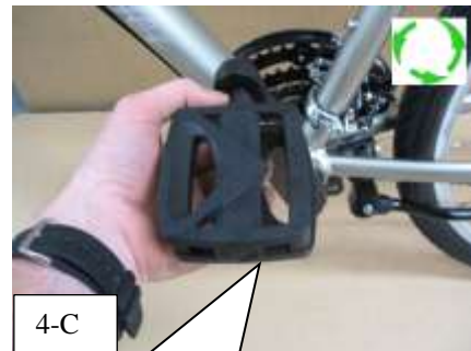
4-C Insert left pedal into left crankarm and turn counter-clockwise.
