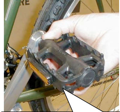
Insert left pedal into left crankarm and turn counter-clockwise.
