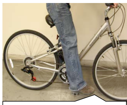
To determine proper saddle height, position right pedal at the bottom of its revolution, aligned with the seat tube. While sitting on saddle, place your heel on right pedal. Your leg should be fully extended.
