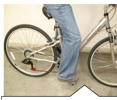
Adjust saddle height if necessary and repeat. Now place the ball of your foot directly over the center of the pedal (normal riding position). This should result in the correct bend at the knee.
